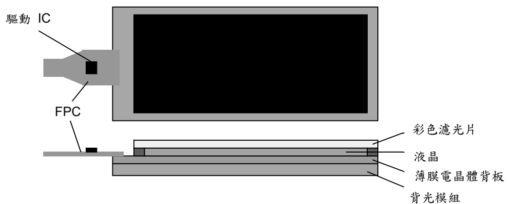
TFF-LCD Module Structure
